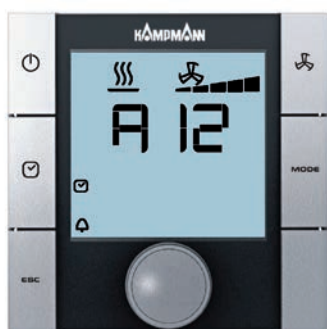
View of "Motor fault" alarm
