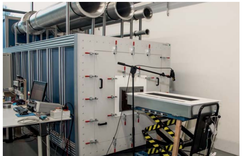
Chamber test rig for air outlet measurements; Kampmann R&D Centre
