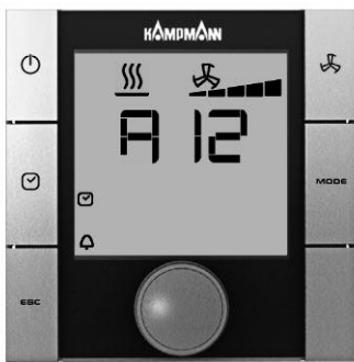
View of "Motor fault" alarm
