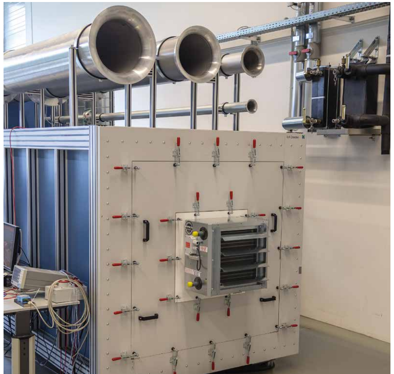
Test chamber for air performance measurements according to DIN EN ISO 5801; Kampmann R & D Centre (FEC)
